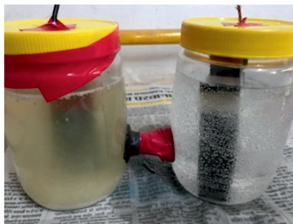
Fig. 5. Bubbling seen in cathode chamber of M.F.C. when sterile dairy effluent in anode inoculated with 5% microbial consortium and 80% of original 30 % hydrogen peroxide solution in cathode chamber.
